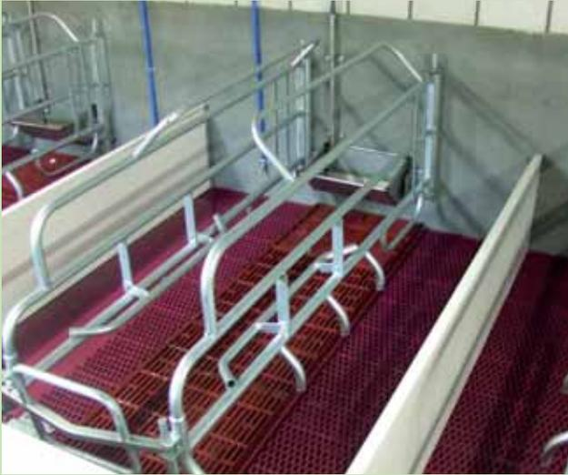
*The combination of slatted floors with a soft coating for the piglets and cast iron grates under the sow is the best farrowing pen floor system.*
